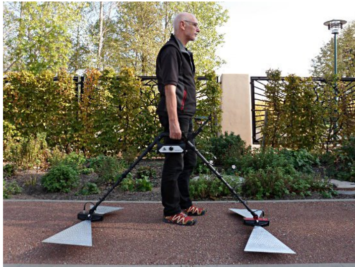
Figure 6.1: Holding the Gepard GPR before starting the scan
