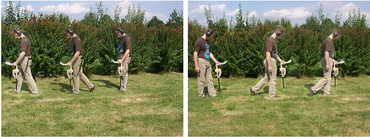
Figure 7.5: "Zig-Zag" scanning in mode Ground Scan
