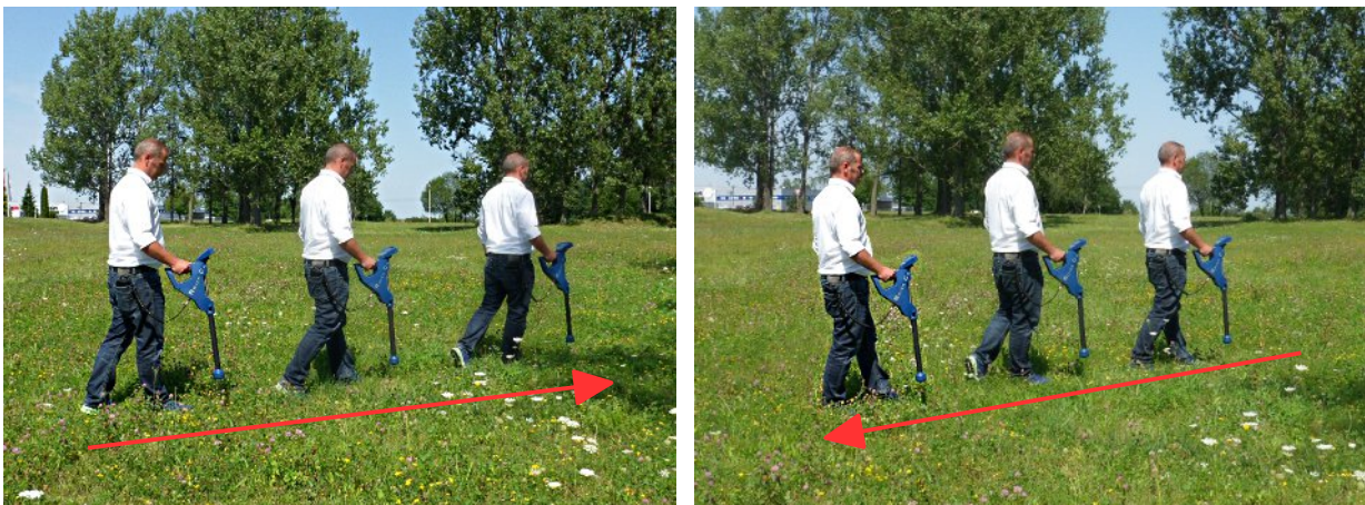
Figure 7.3: "Zig-Zag" scanning in mode Ground Scan
